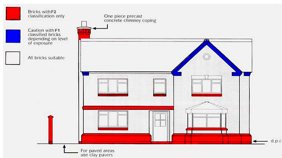
Figure 3.8. Guidelines on where to use different categories of frost resistant bricks in house construction (IBSTOCK 2007, p.2). Guidelines apply to buildings within low exposure zones of the UK.
