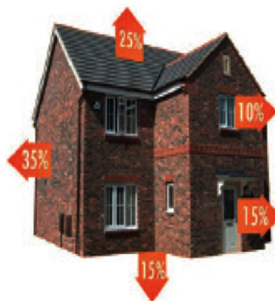
Figure 1.6. Approximate proportions of heat lost from domestic buildings. Note that walls account for around 35%. (DCLG 2006, p.4).
